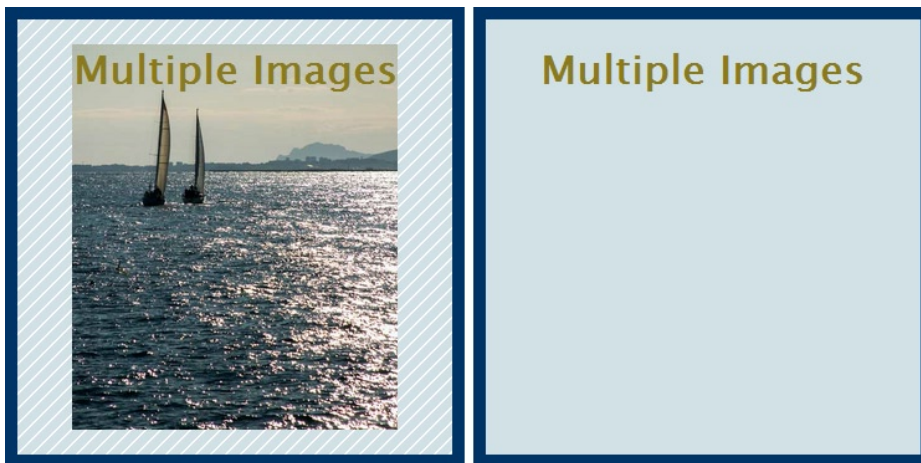
Figure 8-27. Modern browsers support multiple background images, but older versions of IE don't
