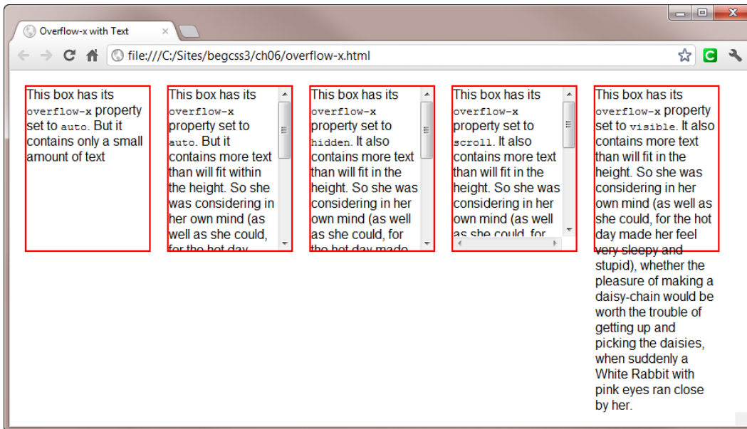
Figure 6-22. Browsers generate a vertical scrollbar for text, even when only overflow-x is set
