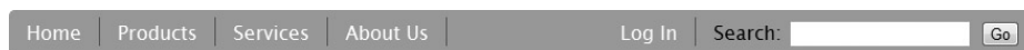
Figure 22-28. Setting the left margin of the Log In link to auto splits the menu into two groups
