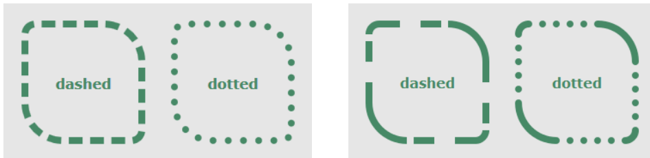
Figure 9-14. Rounded corners on dashed and dotted borders in IE 9 (left) and Firefox 14 (right)
