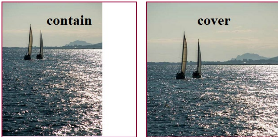
Figure 8-23. The same background image is resized differently without losing its aspect ratio
