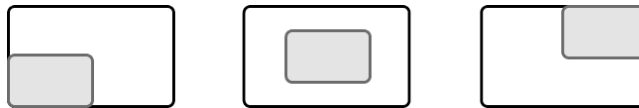
Figure 12-2. A box that animates on hover, showing transform: translate() with one value (the outer box moves from left to right) and two values (the inner box moves horizontally and vertically)
