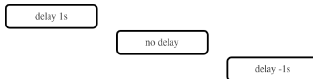
Figure 12-23. We can delay or jump-start the start of a transition using transition-delay . This figure shows 1s into a 3s linear animation.
