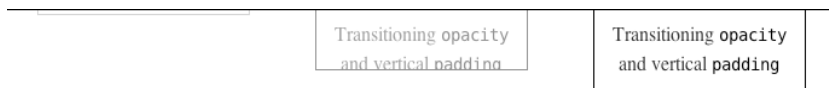
Figure 12-17. Faking transitioning from height: auto; to height: 0; via max-height, plus opacity and padding. For a short transition this is passable.
