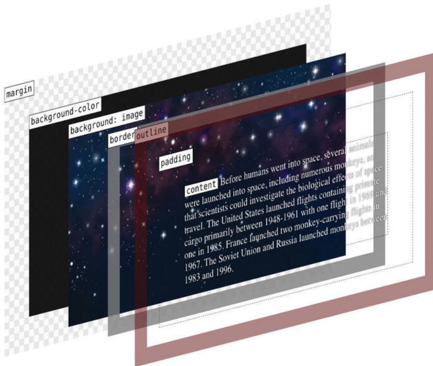
Figure 9-1. A CSS box (including outline), with an exploded view showing how the parts of a block-level box are stacked
