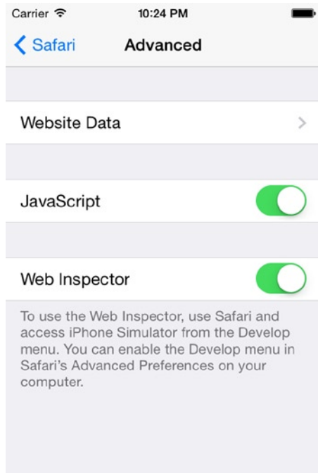
Figure 2-18. Advanced settings for iOS Safari with Web Inspector enabled
