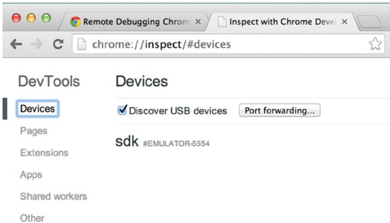
Figure 2-23. Enable device discovery in Chrome
