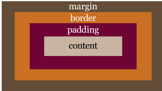
Figure 2.1. A graphic representation of the box model
