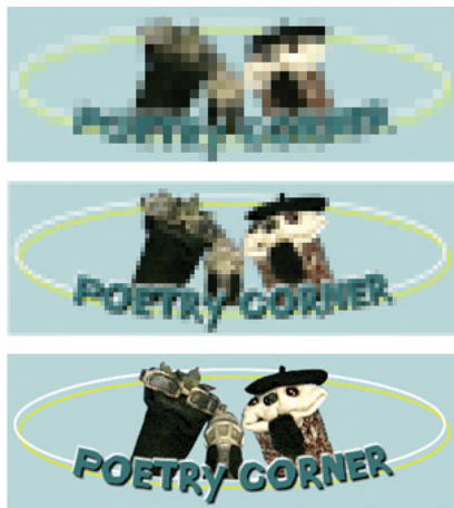
Figure 21-6. Interlaced GIFs display in a series of passes, each clearer than the pass before.
