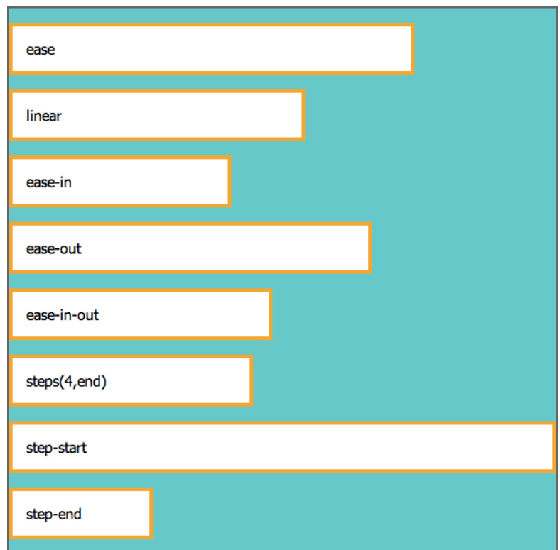
Figure 17-2. In this transition-timing-function demo, the elements reach full width at the same time but vary in the manner in which they get there.
