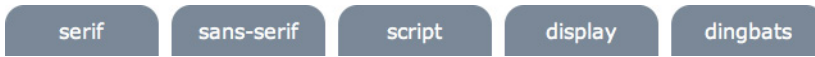
Figure 15-9. The unordered list is transformed into a tab-like menu using CSS alone and no images.
