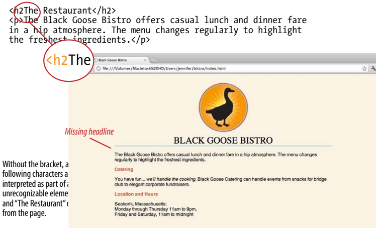
Figure 4-17. A missing end bracket makes all the following content part of the tag, and therefore it doesn’t display.
