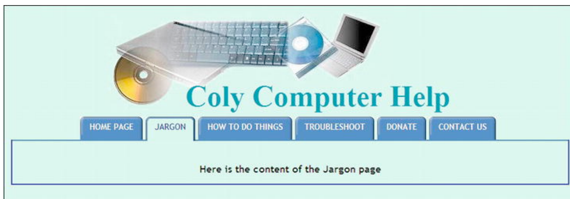
Figure 4-19. The Jargon page has been selected (it is now active) and the tab appears to be part of the page.
