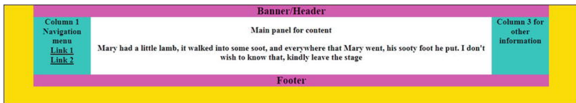
Figure 12-4. A semi-liquid layout with restricted max- and min-widths. This is the best compromise.
