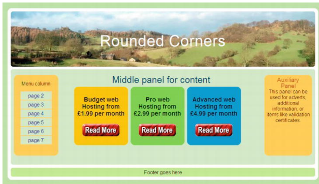
Figure 7-3. A page containing three offers positioned by means of an unordered list. The “Read More” buttons are images with hyperlinks targeting the appropriate pages.
