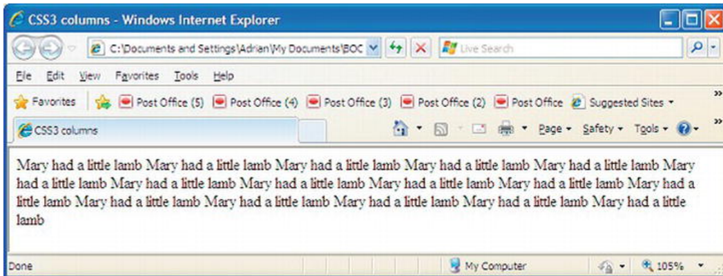
Figure 15-8. The CSS3 multi-column markup fails to display in Internet Explorer 6, 7, 8, 9, and Opera
