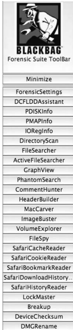
Figure 12.3 The Forensic Suite Toolbar Is a Fast Way to Launch Programs in the Suite
