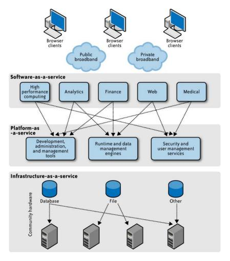
FIGURE 2-4. Architecture for relevant technologies
