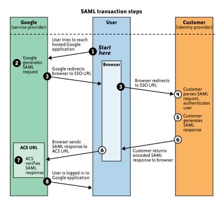
FIGURE 5-3. SSO transaction steps using SAML
