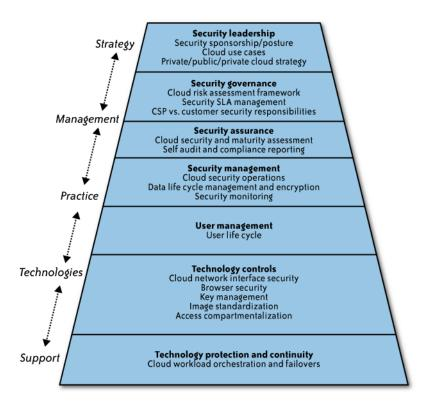
FIGURE 12-4. An enterprise security architecture for cloud computing
