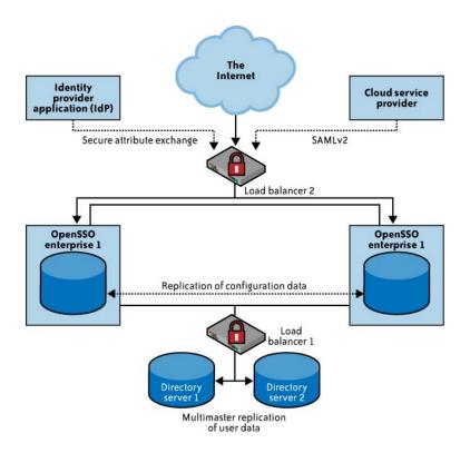
FIGURE 5-7. Identity provider deployment architecture
