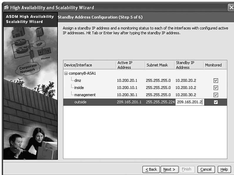
Figure 12-57 Configuring the Standby IP Addresses
