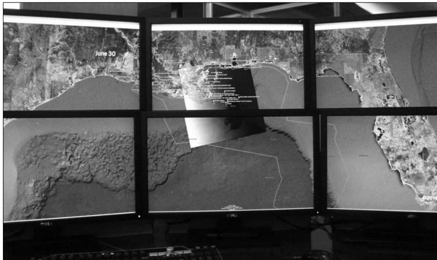
Figure 14-5: A small visualization cluster of three computers, each driving two monitors.
