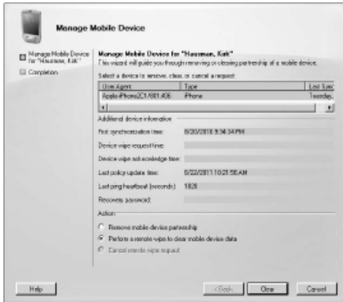
Figure 12-8: The phone wipe inter- face of a common enterprise collabora- tion suite.
