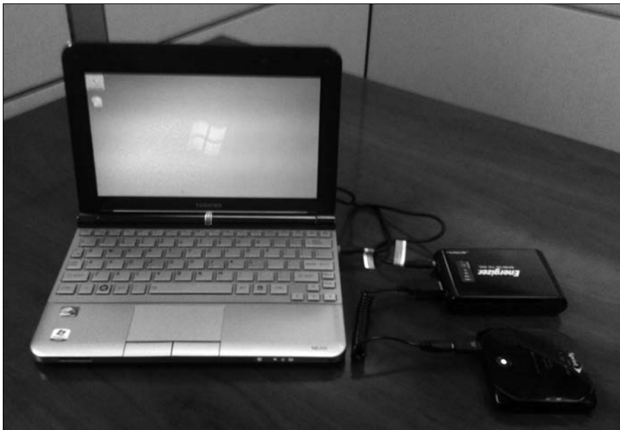
Figure 12-5: A power pack the size of a small deck of cards can add several hours of operation to a netbook and charge various other mobile devices while you're on the road.
