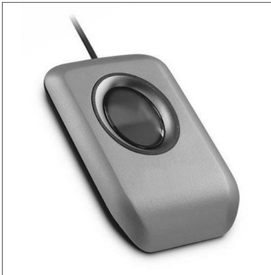
Figure 7-2: An example of a USB fingerprint biometric reader provided by Engineersoft through the Wikimedia Commons.
