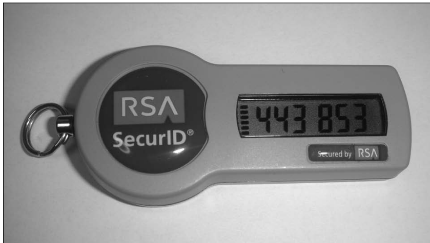
Figure 7-1: An RSA SecureID informa- tional access token.
