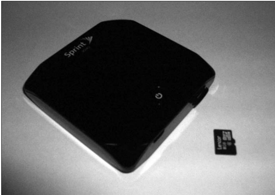
Figure 12-2: A 3G/4G cellular data link providing a Wi-Fi hotspot for WLAN access between up to five devices.
