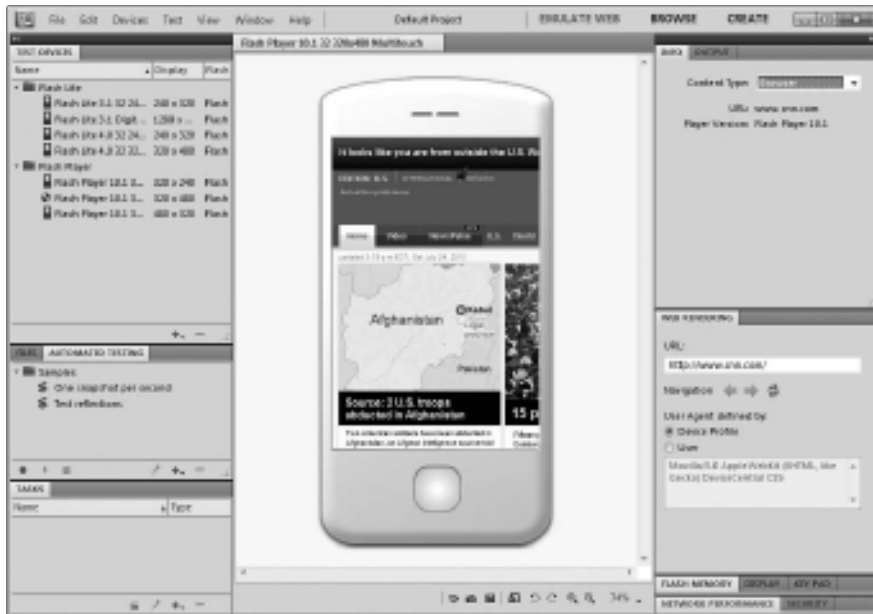
Figure 12-6: A mobile device emulator displaying a popular news Web site using the designated device, browser, and version of Flash player.
