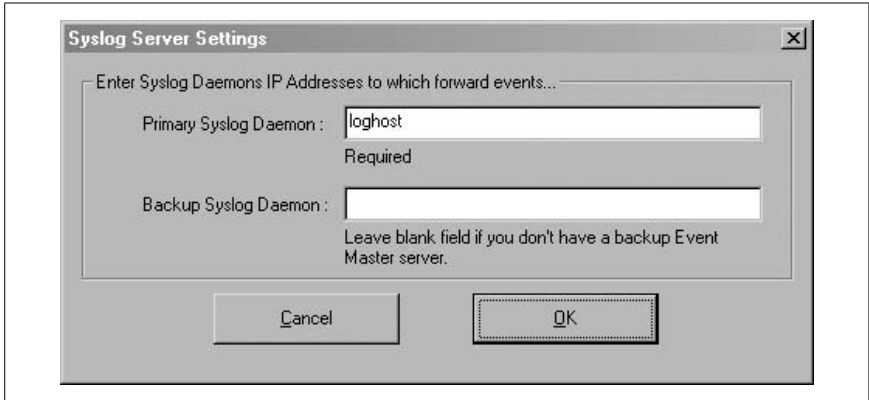
Figure 8-8. Specifying a primary and backup syslog server
