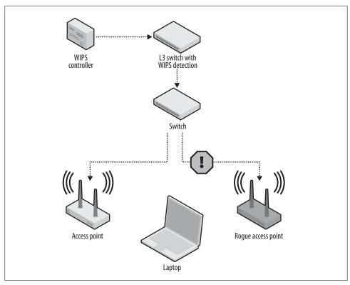
Figure 2-8. A wireless intrusion prevention system (WIPS)
