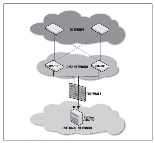
Figure 3-7. NetFlow collection at DMZ backbone routers
