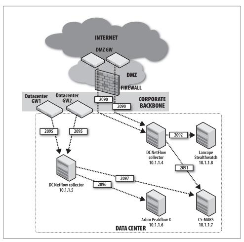
Figure 6-14. Copying NetFlow to other devices with flow-fanout
