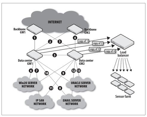
Figure 6-8. A data center network design—demonstrating choke point collection and sensor load balancing
