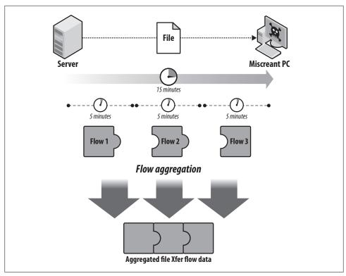
Figure 3-10. Flow aggregation of a file transfer
