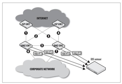
Figure 6-6. Placement of NIDS to inspect a DMZ with redundant ISP connections
