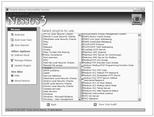
Figure 4-2. Nessus scan options for SCADA systems
