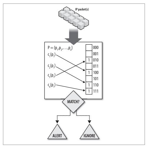
Figure 6-1. Pattern matching methodology used by a NIDS
