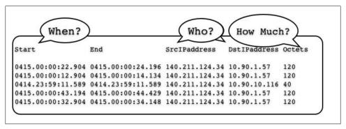
Figure 3-4. An example of NetFlow (http://www.cisco.com/en/US/docs/net\_mgmt/netflow\_collection \_engine/3.0/user/guide/nfcform.html)
