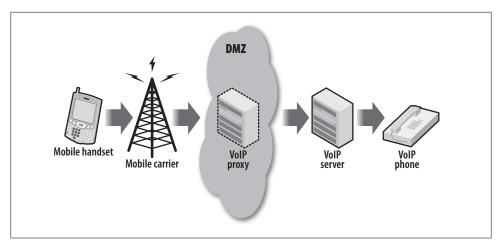
Figure 8-1. A VoIP proxy which provided a gateway between the mobile carrier's network and the VoIP server, but presented risk to Ansalya's network
