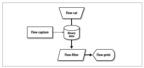
Figure 3-8. Basic flow-tools components
