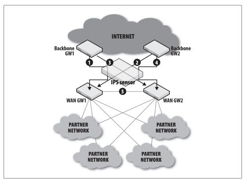
Figure 6-9. Sensor placement and connectivity for extranet
