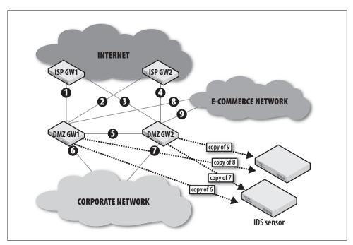
Figure 6-7. Configuration of NIDS to accommodate a more complex DMZ network
