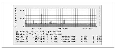
Figure 3-11. SNMP queries for network interface data graphed over time with MRTG
