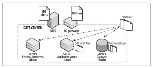
Figure 4-7. Where to collect logs for SAP R/3 monitoring
