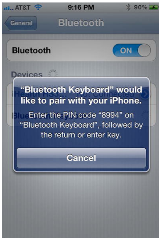
Figure 3–20. To pair your iPhone to a Bluetooth keyboard, make the keyboard discoverable, find it in the iPhone's Bluetooth settings, and then tap the keyboard name. To consummate the pairing, you'll need to type in a random passkey created by the iPhone.
