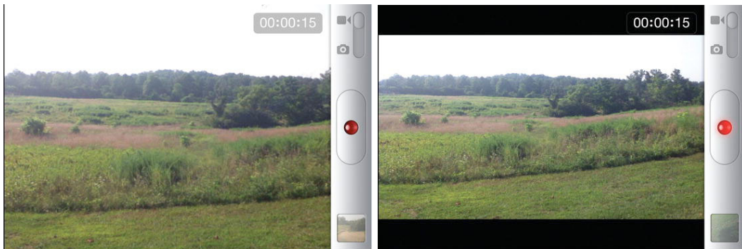
Figure 13-6. The video-recording screen shows the time elapsed while recording. Double-tap the screen to enter 16:9 aspect ratio.
