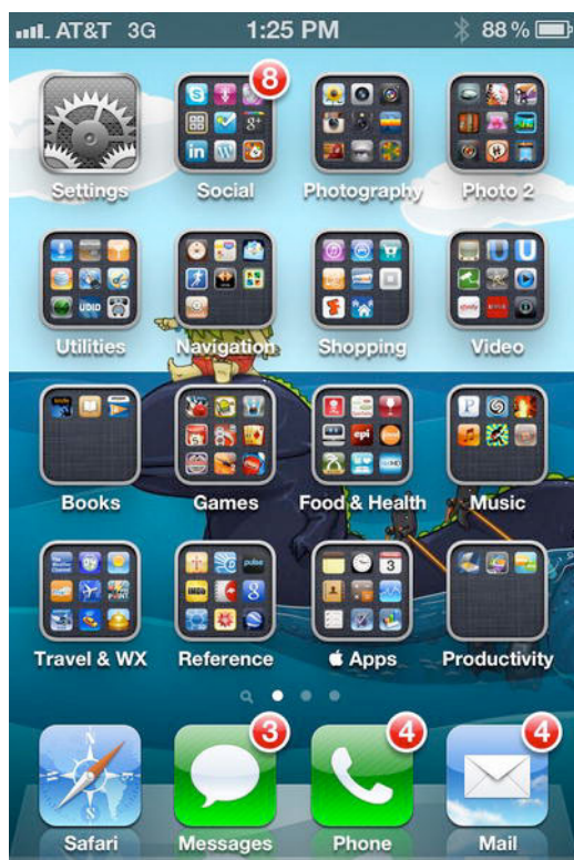
Figure 5–5. On the status bar at the top of this image, you see the bars indicating the cellular network signal strength (four bars), the carrier name (AT&T), and the type of network the iPhone is connected to (3G).
