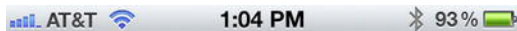
Figure 5–1. The three arcs shown here indicate a strong Wi-Fi connection. Blue arcs indicate the strongest connection. Black arcs mean a weak connection. Very light gray arcs show the worst connection.
