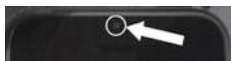
Figure 3–3. You can “see” the iPhone's IR light from its proximity sensor if you own a digital camera. Its IR beam is visible to the camera's detector. Make sure to cover the iPhone's screen when you take the photograph, because it's bright and the IR light is dim.
