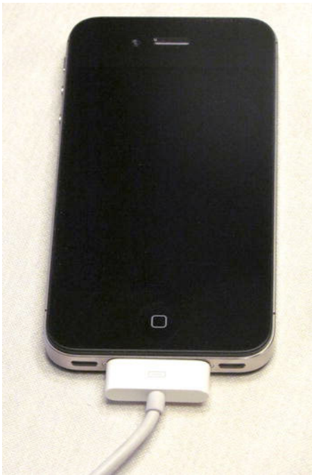
Figure 1-5. Plug the USB-to-dock connector cable into the iPhone with the rectangle mark facing you.
