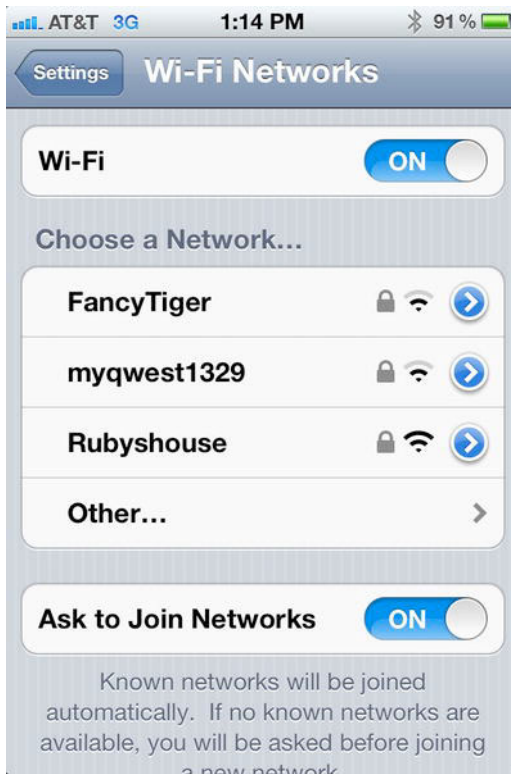
Figure 5–2. Set Wi-Fi to On to connect to local networks. A lock icon next to a network name indicates that you must use authentication to connect.
