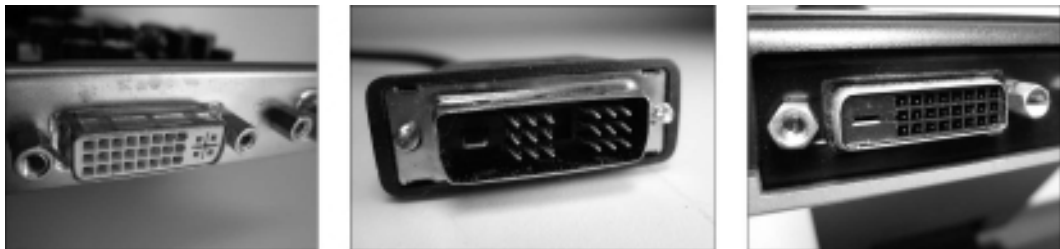
Figure 9-4: A DVI port on a video card (left), cable connector (middle), and monitor (right).
