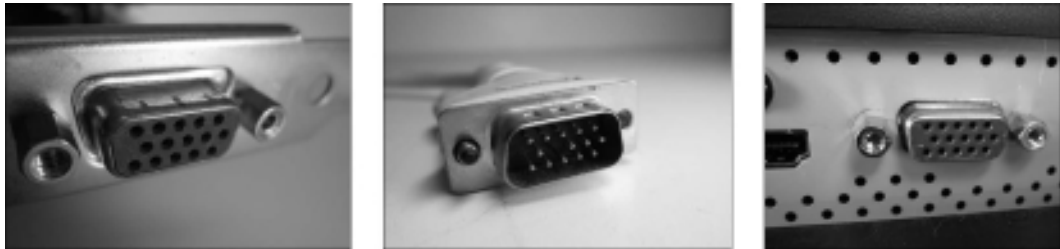
Figure 9-3: A VGA port found on a video card (left), cable connector (middle), and monitor (right).
