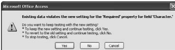
Figure 4-3: If Access finds an empty value, then it stops the search and asks you what to do about it. You can keep your changes (even though they conflict with at least one record)—after all, at least new records won't suffer from the same problem. Your other option is to reset your field to its more lenient previous self. Either way, you can track down the missing data by performing a sort on the field in question (page 97), which brings empty values to the top.
