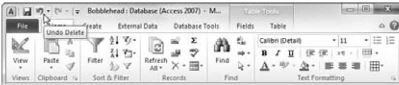
Figure 1-11: The Undo command appears in the Quick Access toolbar at the top left of the Access window, so it's always available.
