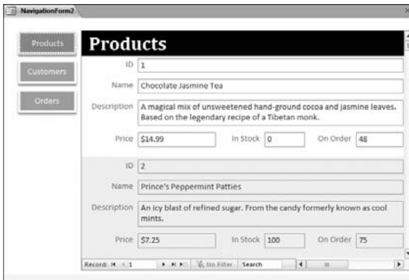
Figure 14-18: This navigation form uses several tricks to improve its appearance. It has no header, the navigation buttons are artfully styled, and the navigation subform uses anchoring so it expands to fill the available space. You can find this example, along with all the navigation forms in this chapter, on the Missing CD page ( www.missingmanuals.com/cds ).
