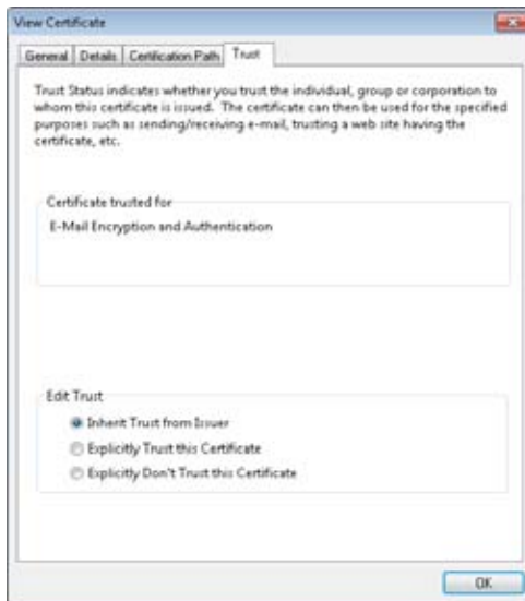
Figure 14-18 Use the Trust tab to configure the trust relationship for the certificate.
