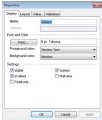
Figure 27-9 You can use the Properties dialog box to modify the properties of a control.
