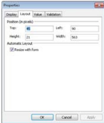
Figure 27-10 Use the Layout tab to set the position and size of a control.
