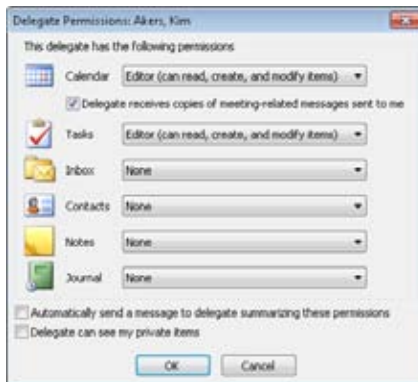
Figure 21-5 Use the Delegate Permissions dialog box to control the visibility of private items.
