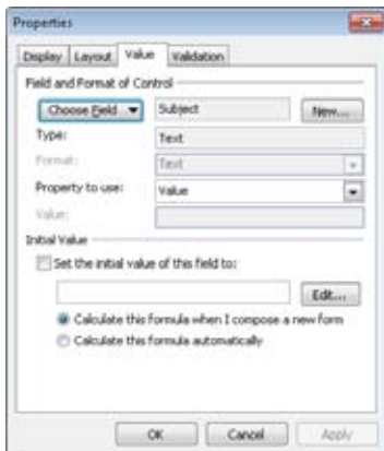
Figure 27-11 Use the options on the Value tab to set the field and format for a control.
