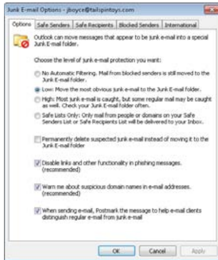
Figure 12-1 Use the Junk E-Mail Options dialog box to configure Outlook 2010 quickly to filter unwanted messages.
