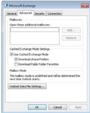
Figure 39-4 Use the Advanced tab to configure additional mailboxes, Cached Exchange Mode, and offline file settings.
