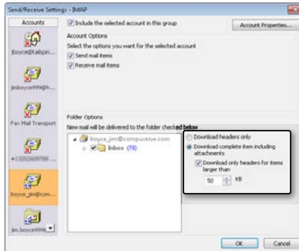
Figure 15-6 You can specify a message size limit to control connect time and mail volume.
