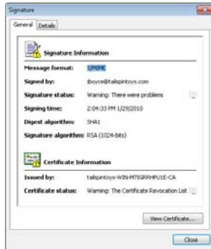
Figure 14-23 Use the Signature dialog box to view additional properties of the signature and to access the certificate.
