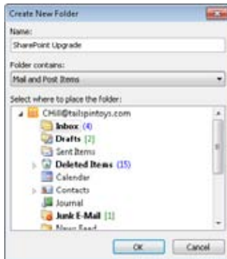
Figure 29-3 Use the Create New Folder dialog box to specify folder type, location, and other properties of a new folder.
