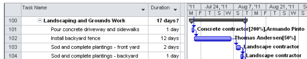
Figure 10-13 Assignment units other than 100% are shown next to the relevant Gantt bars.
