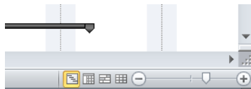
Figure 1-13 Use the Zoom slider to adjust the timescale to more or less detail.
