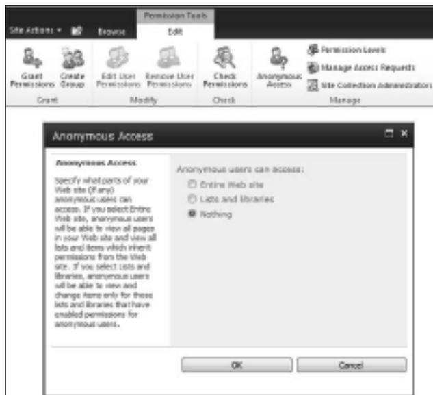
Figure 2-1: Setting Anonymous Access at the site level.
