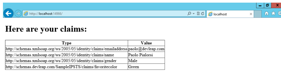
FIGURE 20-5 The output of the Default.aspx page after authentication with a sample user.
