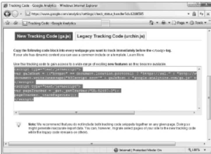
Figure 1-11: The Google Analytics code is lean and concise, requiring just a few lines. That's because it links to a file on Google's Web servers to get the real tracking code. Select all the code displayed, and then copy it to your clipboard (you do this in most browsers by right-clicking the selected text, and then choosing Copy).
