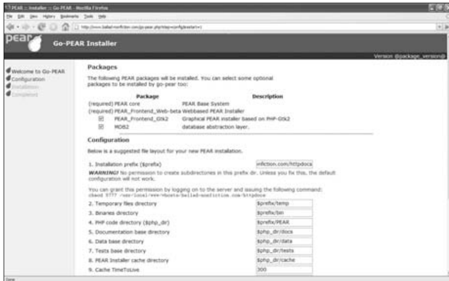
Figure 2-2: The configuration screen warns that the script doesn't have enough permissions to install PEAR.
