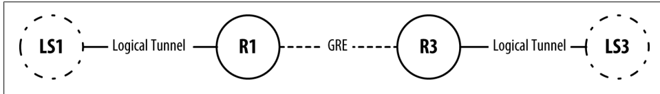
Figure 7-14. Tunnel Services Case Study: Logical End-to-End Connectivity.
